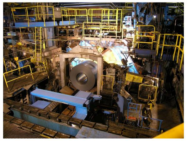
Hot Strip Mill Downcoilers and Coil Handling for Sale Mfr: SMS Age: 1990 Quantity: 2 Identical Design: Retractable Hydraulic 3 Wrapper Roll Strip Properties: Thickness: .500" - .061" [ 12.7 - 1.57mm ], Width: 61" - 24" [ 1549 - 609mm ], Weight: 58,000#, 1100 PIW, 2000 FPM [ 609MPM ] Drive Motors: Mandrel - 1000HP 430-1290rpm 500VDC, Wrapper Rolls [3] -100HP Frame MD808 Strip Mill Capacity: 250,000TPM
